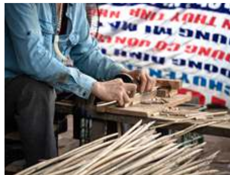
Cutting the stems of bamboo into length of 20-21cm.
