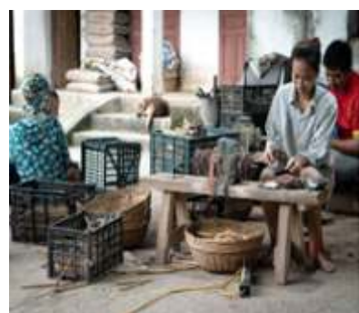
Using sandpaper to smooth bamboo outer surface
